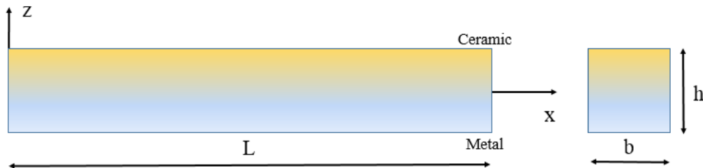
Figure 6.1 Geometry of FG beam
