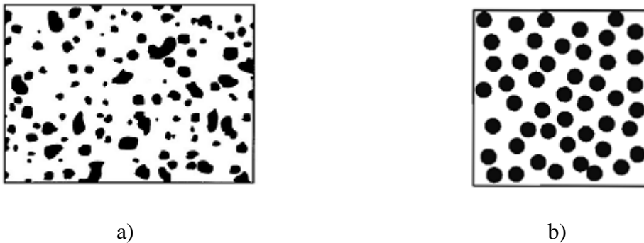
Figure 2.1 Particulate and fiber composite materials
